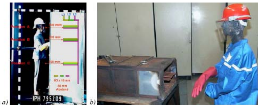
Picture 4: Test structure as per IPH Procedure.
