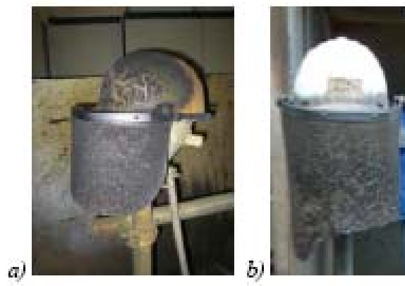
Figure 6: Face shield subjected to 10 kA for 1 second in two different test procedures and positioned 300 mm from the electric arc (left IPH Berlin, position A, right RWE Eurotest).
